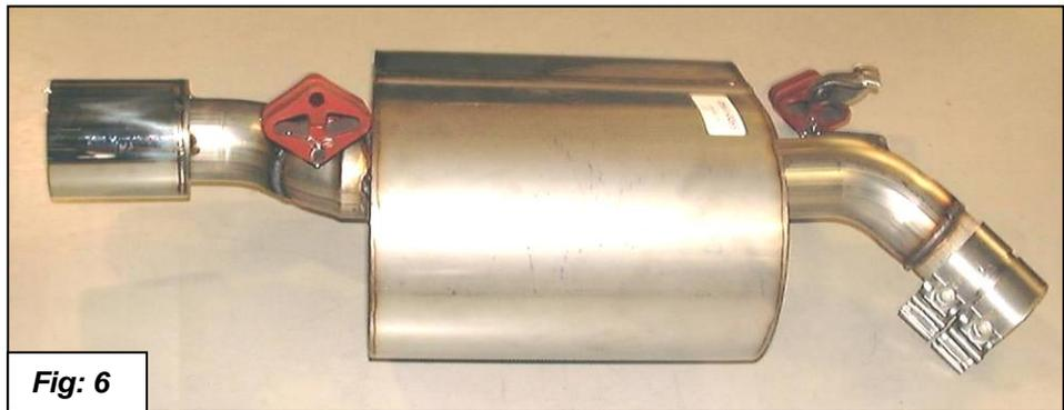
8. Install the hangers, mounts and clamps onto the Dinan mufflers as shown in figures 6 and 7. Secure the hangers to the rods with a cotter pin on each side of the hanger.
