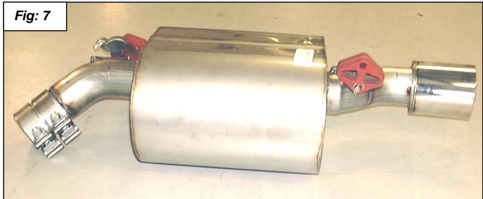
9. Install each muffler by sliding the clamps over the ends of the pipes. Attach the hangers to the car with the stock bolt and nut in the front and push the hanger over the stock rod in the rear as shown in figures 8 and 9.
