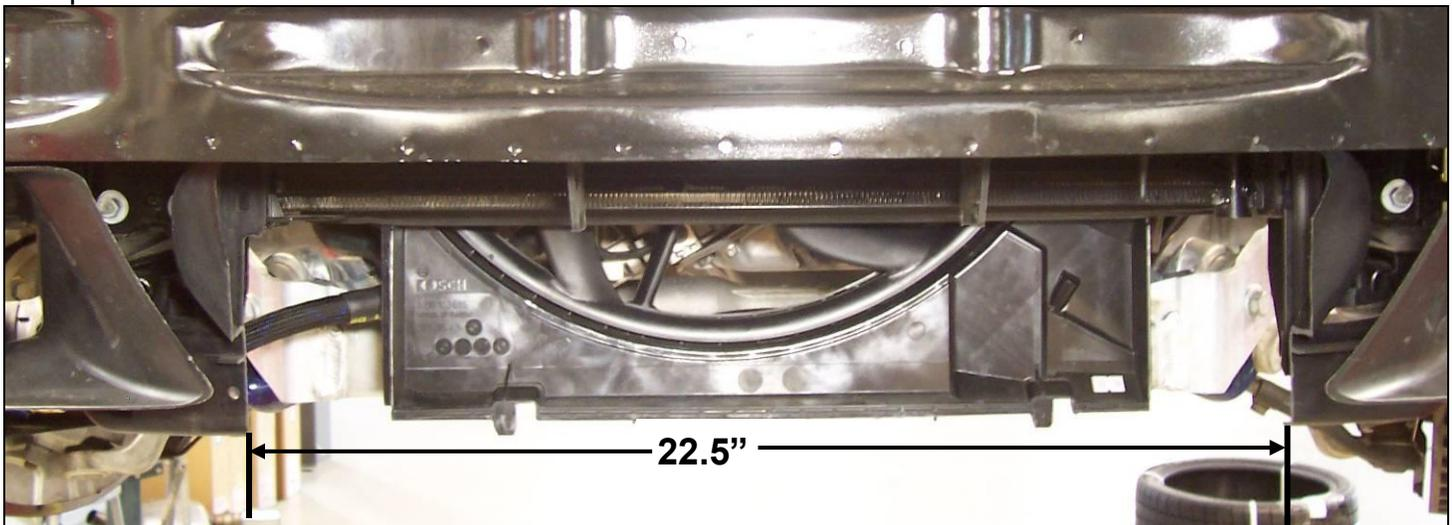
6. The two photos below show where the Intercooler ends meet the mounting screw areas. You may be able to trim less than the photo shows, as this was the prototype car install. I purposely overexposed the photo so the "hard to see" black plastic is much more visible. I have circled the areas of contact that require trimming.
