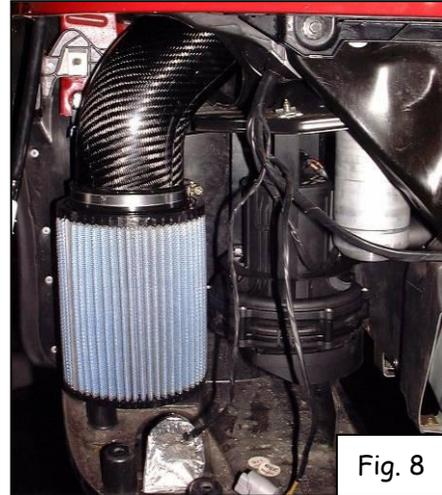
21. See Figure 8: Install the Air Filters onto the intake tubes with the supplied hose clamps. Make sure the filters don't interfere with the mounting of the front bumper.
