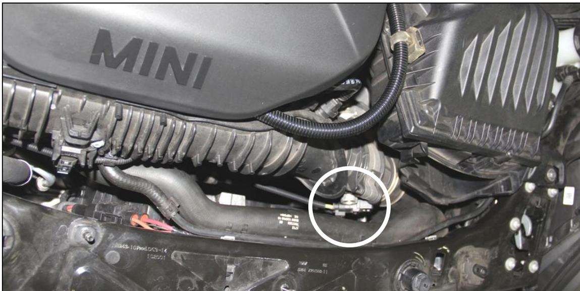
6. Disconnect the wiring harness from the pressure sensor.
